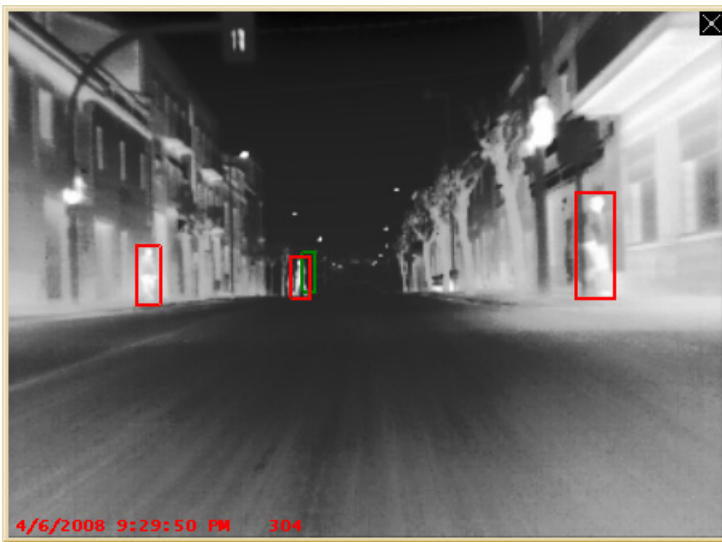
Fig. 2. An infrared snapshot of pedestrians obscured by background thermal radiation and the corresponding time series the metric
