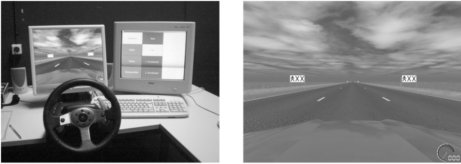
Fig.1. Experimental setup on the left, the drivers view on an indicated lane change on the right
